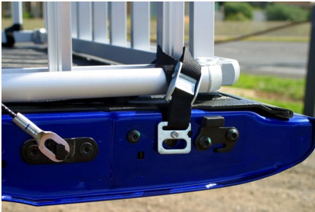
Toyota Installation--It's OK to loop around the ramp rail as well. Install once--don't remove.
