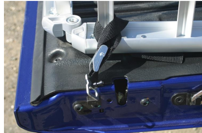
Toyota Installation--It's OK to loop around the ramp rail as well. Install once--don't remove.
