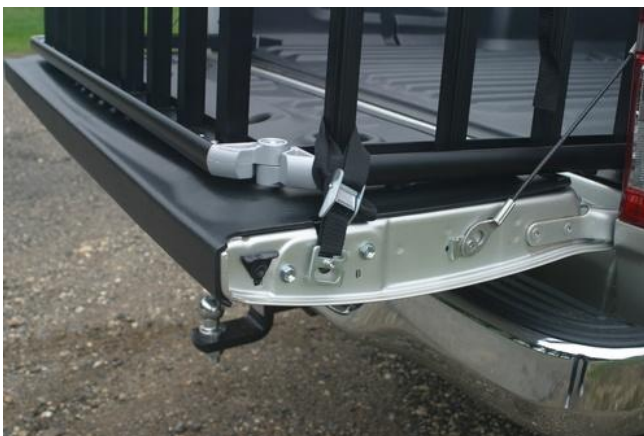
Most "Post & Latch" full-sized truck installation. It's OK to loop around the ramp rail as well. Install the hardware once; it will be in the perfect location the next time you use the ReadyRamp.
