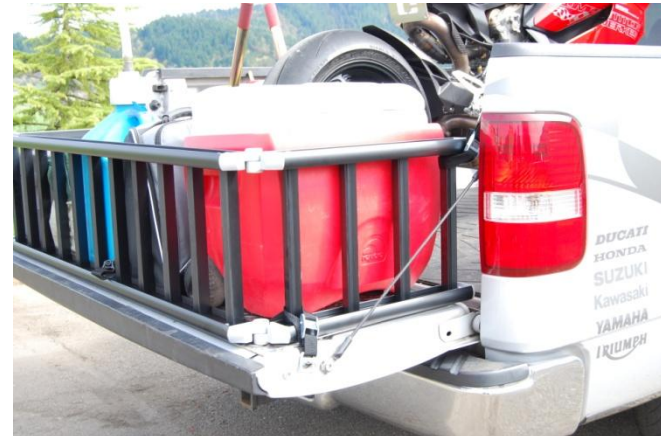
Most "Post & Latch" full-sized truck installation. It's OK to loop around the ramp rail as well. Install the hardware once; it will be in the perfect location the next time you use the ReadyRamp.
